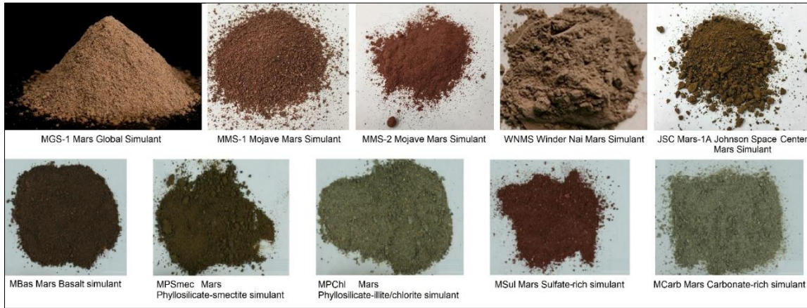
Fig 1: Comparison images between Martian simulants (photo: CLASS Exolith Lab and CSM Planetary Simulant Database, [18, 19].
