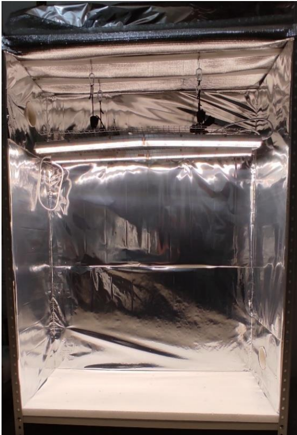
Fig 9: Growth chamber with thermally insulated panels and covered with film reflective.
